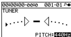
**3** To turn off the tuner, press the [EXIT] button.
