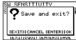
To save your settings, press the [ENTER] button; to return to the SW SENSITIVITY screen, press the [EXIT] button.
