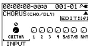
**3** Use the CURSOR [◀] [▶] buttons and the dial to adjust the send level of each track.
