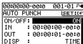
**3** Use the CURSOR [▲][▼] buttons to move the cursor to "ON/OFF," and turn the dial to choose "ON."
