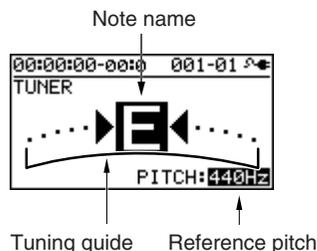
The tuning guide indicates the difference between the input pitch and the displayed note name. If the difference between the input and the correct pitch is within  $\pm 50$  cents, the tuning guide shows the amount of difference.
